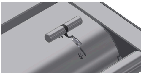
Figure 8: While in manual mode, handle has to be in lock position.
